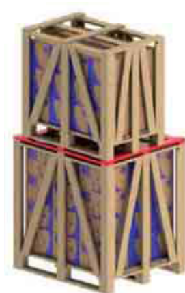
Figure 5.5 - Use of additional battens for stacking
