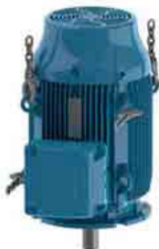
Figure 4.17 - Install the second pair of eyebolts
