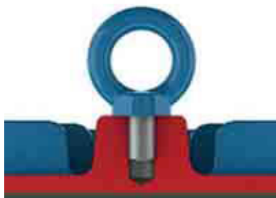
Figure 4.1 - Correct tightening of the eyeboll
