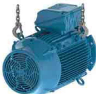
Figure 4.19 - Final result: motor placed in horizontal position
