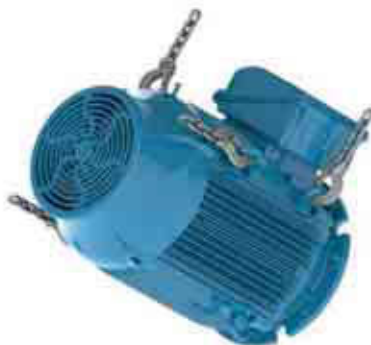
Figure 4.18 - Motor is being rotated to horizontal position
