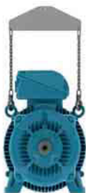
Figure 4.6 - Use of a spreader beam for lifting
