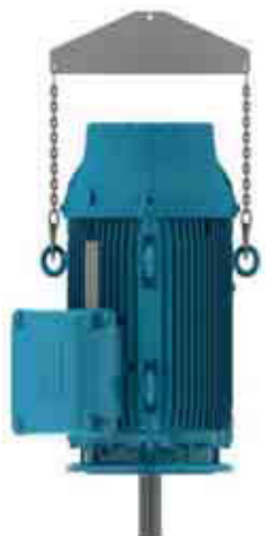
Figure 4.7 - Lifting of vertical mounted motors
