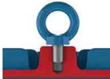
Figure 4.2 - Incorrect tightening of the eyeboll
